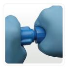
While holding the CryOmega® device with one hand, firmly grasp the knob at the end of the device with the other hand.
